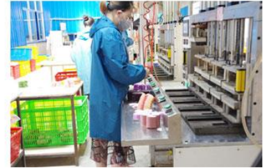
Step 4: Shape the petals using automatic setting machine.
