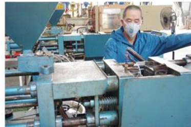
Step 5: Operate automatic plastic ejection machine for stalk by manipulator
