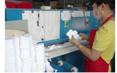
Step 4: Shape the petals using automatic setting machine.
